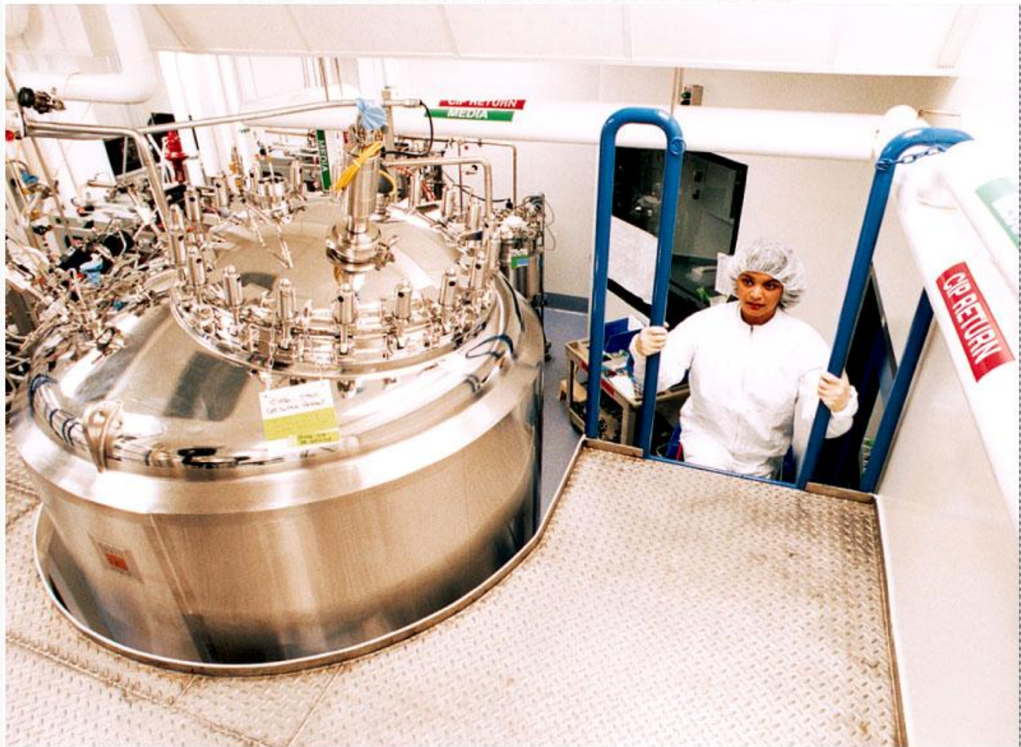
Fig. 24.30 A cell culture vessel used to mass-produce Pharmaceuticals.
